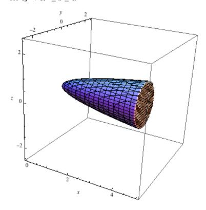
Next, let D be the projection of E onto the yz-plane by considering its widest part (at x=4), so the projection will be  $4y^2+4z^2\leq 4$ , or  $y^2+z^2\leq 1$  (i.e. a circle!). Using polar coordinates in the yz-plane, we can define  $y=r\cos\theta$  and  $z=r\sin\theta$ , where we will bound r by 1 (the radius is 1) and every angle should be considered,  $0\leq\theta\leq 2\pi$ . Then we have
