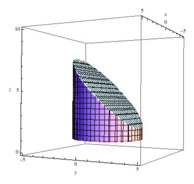
The lower plane is at 1, and the upper plane is y+z=5, then we can see  $1 \le z \le 5-y$ , and solving for y in the equation of the cylinder,  $x^2+y^2=9$ , we find  $-\sqrt{9-x^2} \le y \le \sqrt{9-x^2}$ . Finally, since the radius of the cylinder is 3 and it's centered at (0,0) in the xy-plane, we see  $-3 \le x \le 3$ , so we can set up the integral:
